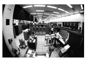
now comprised five linked **IBM 7094s**, five **IBM 2361 Core Storage Units**, and two **IBM 1460s**. The **IBM 2361** was the largest computer memory ever built by the company and consisted of nearly **20 million doughnutshaped ferrite cores**, capable of storing 2.6 megabytes of data.
