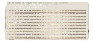
Frequently in data processing applications fewer than 80 data columns were used with the remaining columns holding control information about the card itself.
