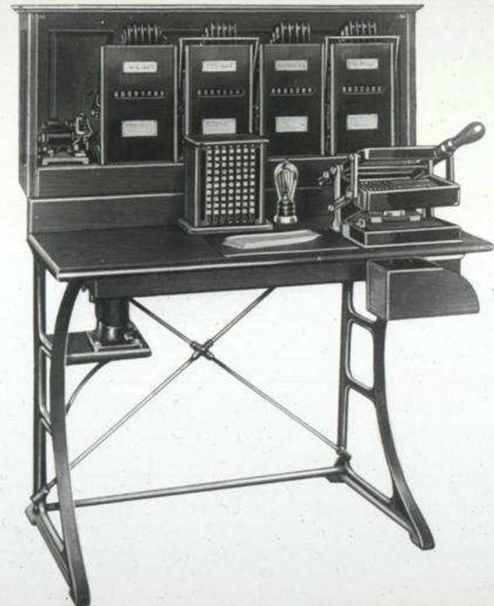
Original Electric Tabulating Machine For Railroad and Commercial Accounting
